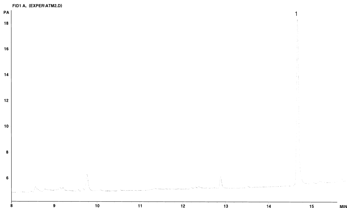
Fig. 2. Gas chromatogram obtained from the analysis of a sample bulb by SPME–GC–FID ( 1.9 \text{ mg/m}^3 controlled atmosphere of tetrachloroethylene). (1) Tetrachloroethylene.
